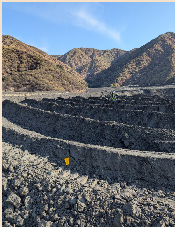
A worker collects soil samples as NASA aims to find backfill that meets soil cleanup standards and can support revegetation following cleanup activities.
