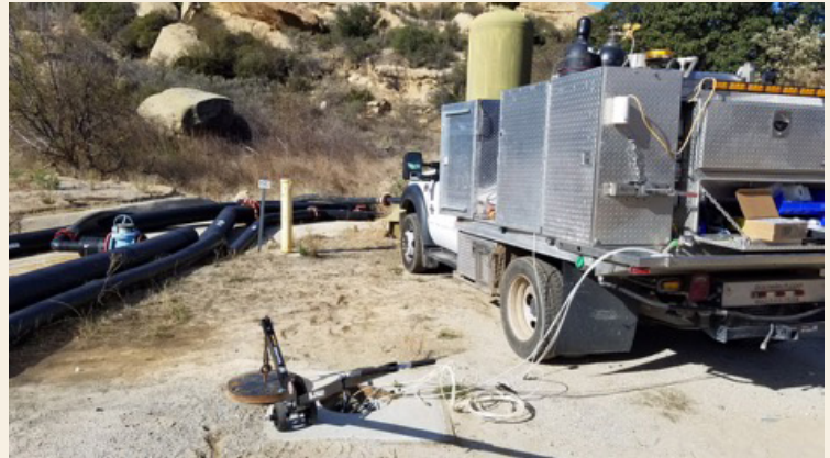
NASA's groundwater characterization work included extensive sampling of groundwater. The above photo shows groundwater sampling of a flush mounted multi-port well in the R2 Ponds area in NASA Area II.
