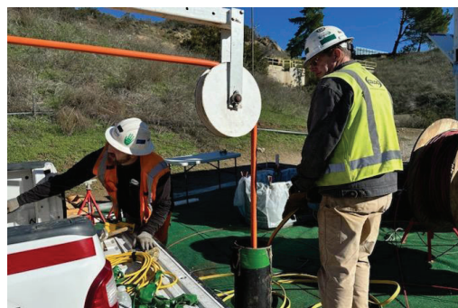
Groundwater crews conduct packer testing and depth discrete groundwater sampling at ND-160, a 1,000-foot deep data gap well located near Alfa Test Stand 2 in NASA's Area II.
